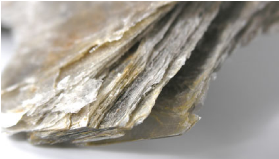
Figure 8.47 Mica Exhibits One-Plane of Cleavage—Sheets. Image is used under a CC BY: Attribution license.
