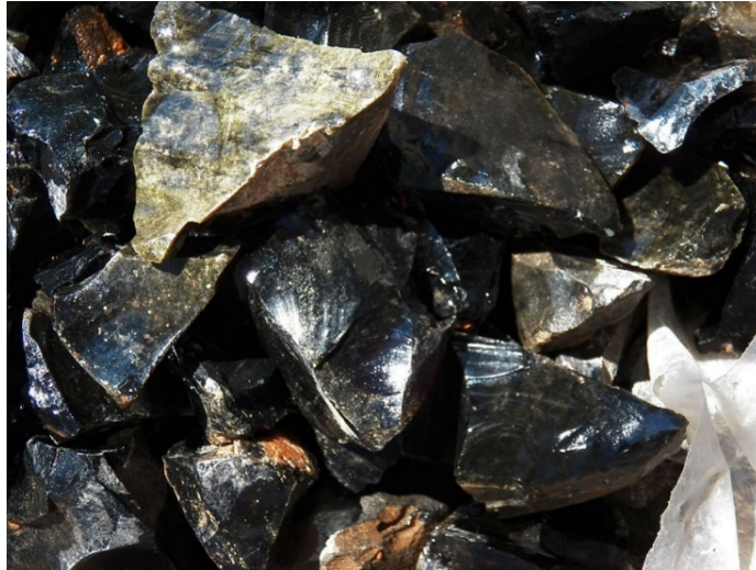
Figure 9.7 Close-Up of an Obsidian Sample. This Extrusive Rock Cooled Quickly from Felsic Lava. Jeremy Patrich is used under a CC-BY 4.0 license.
