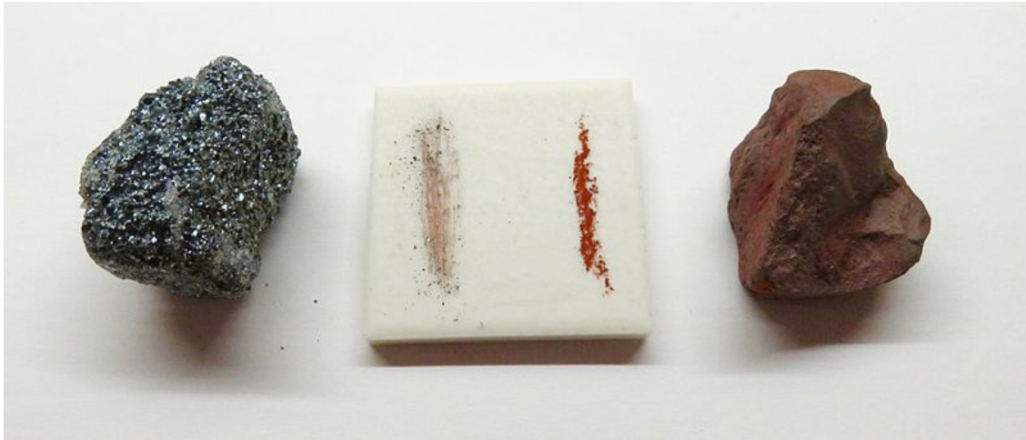
Figure 8.44 Hematite Leaves a Reddish-Brown Streak on a Ceramic Plate Whether the Hematite has a Metallic Luster or an Earthy Luster. Image by is licensed under a Attribution-Share Alike 4.0 International license.
