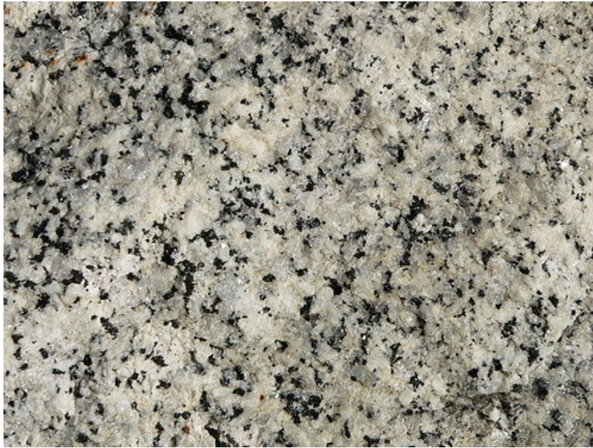
Figure 9.6 Close-Up of a Granite Sample. This Sample, it is Easy to See & Identify the White & Black Crystals, so This Specimen Cooled Slowly. Jeremy Patrich is used under a CC-BY 4.0 license.
